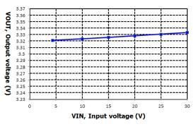
VIN=4.3V to 30V, VOUT=3.3V @ IOUT=10mA
