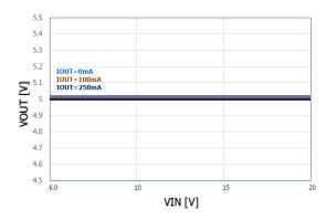
VIN=6.0V to 20V, VOUT=5.0V @ IOUT=0A/100mA/250mA  $\label{eq:VIN} VIN \ \ vs. \ \ VOUT$
