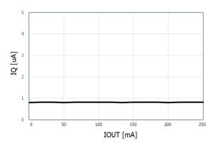
VIN=6.0V, VOUT=5.0V @ IOUT=250mA per 10mA step  ${\rm IOUT\ vs.\ IQ}$
