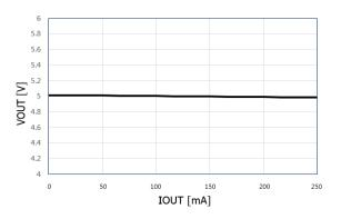
VIN=6.0V, VOUT=5.0V @ IOUT=250mA per 10mA step IOUT vs. VOUT
