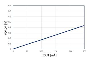
VIN=6.0, VOUT=5.0V @ IOUT=250mA per 10mA step IOUT vs. VDROP
