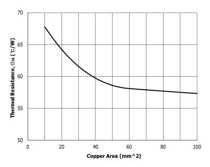
The maximum allowable power dissipation is also influenced by the ambient temperature. With the  $\theta_{JA}$ -Copper plane area relationship, the maximum allowable power dissipation could be evaluated with respect to the ambient temperature. As shown in graph, the higher copper plane area leads  $\theta_{JA}$ . And the higher ambient temperature leads lower maximum allowable power dissipation.
