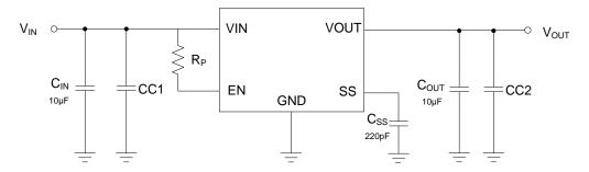
Fig. 1. Application with Decoupling Capacitor, CC1 & CC2
