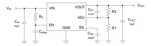
Fig. 3. Application with Delayed Start-Up
