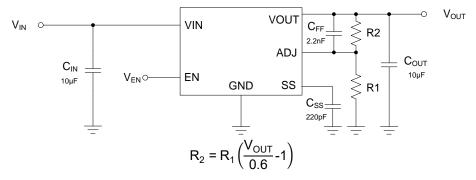
Fig. 4. Application for Adjustable Output Voltage
