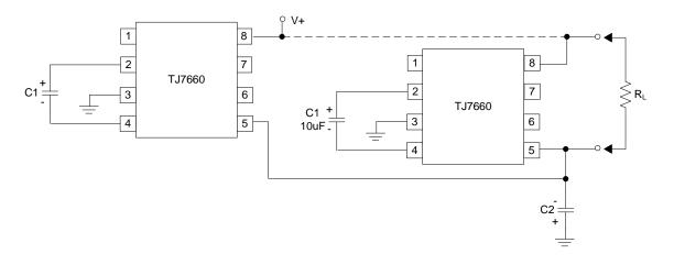
Figure 15. Paralleling Devices
