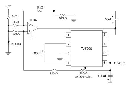
Figure 22. Regulator the Output Voltage
