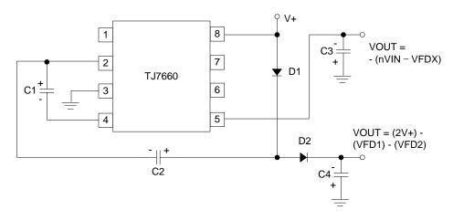
Figure 20. Combined Negative Voltage Converter and Positive Doubler
