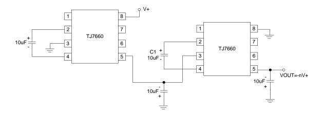
Figure 16. Cascading Devices for Increased Output Voltage
