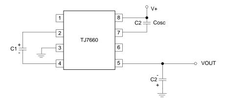
Figure 18. Lowering Oscillator Frequency
