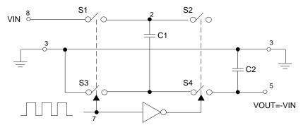
Figure 12. Idealized Negative Voltage Converter
