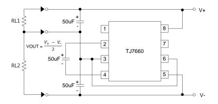
Figure 21. Splitting a Supply in Half
