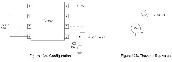
Figure 13. Simple Negative Converter
