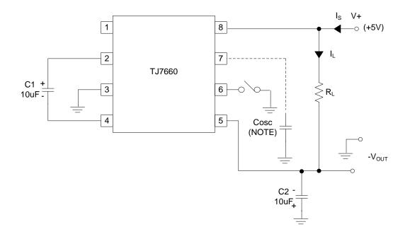
Note. For large values of Cosc (>1000pF) the values of  $C_1$  and  $C_2$  should be increased to 100uF.
