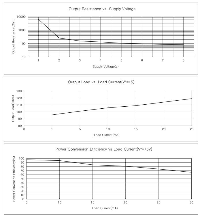
Note. These curves include in the supply current that current fed directly into the load  $R_L$  from the V<sub>+</sub> (See Figure 11). Thus, Approximately half the supply current goes directly to the positive side of the load, and the other half, through the LM7660, to the negative side of the load, Ideally,  $V_{OUT}=2V_{IN}$ ,  $I_B=2I_L$ , so  $V_{IN} \times I_B=V_{OUT} \times I_L$
