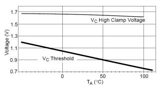
Figure 11. Vc Threshold and High Clamp
