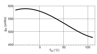
Figure 16. Error Amplifier Transconductance vs. Temperature
