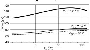
Figure 13. Shutdown Delay vs. Temperature
