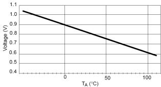
Figure 12. Shutdown Threshold vs. Temperature
