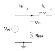
Figure 26. Boost Circuit Effective Input Filter
