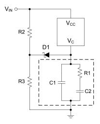
Figure 28. Current Limiting using a Diode Clamp
