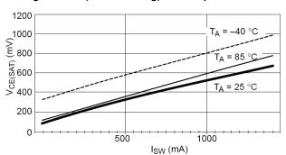
Figure 5. V<sub>CE(SAT)</sub> vs. I<sub>SW</sub>
