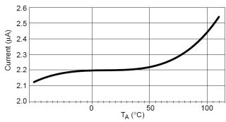
Figure 17. Switch Leakage vs. Temperature
