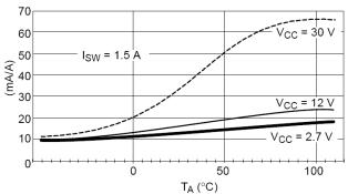
Figure 4.  $\triangle Icc/\triangle Ivsw$  vs. Temperature
