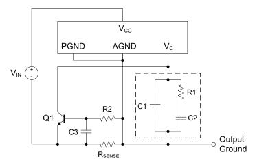
Figure 29. Current Limiting using a Current Sense Resistor
