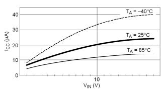
Figure 15. I<sub>CC</sub> vs. V<sub>IN</sub> During Shutdwon
