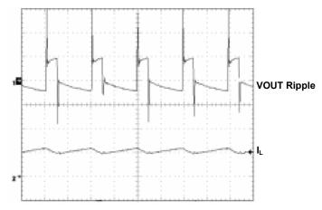
Figure 27. Typical Output Voltage Ripple
