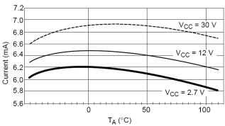
Figure 3. I<sub>CC</sub>(No Switching) vs. Temperature
