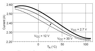
Figure 9. Current Limit vs. Temperature
