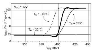
Figure 8. Switching Frequency vs. V<sub>FB</sub>
