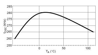
Figure 7. Switching Frequency vs. Temperature
