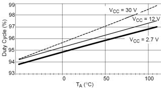
Figure 10. Maximum Duty Cycle vs. Temperature
