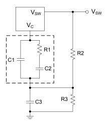
Figure 30. Technique for Increasing Slope Compensation
