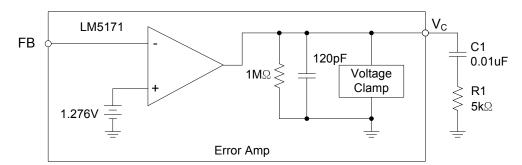
Figure 21. Error Amplifier Equivalent Circuit
