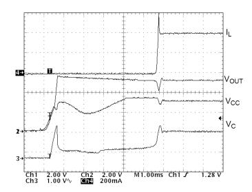
Figure 22. Startup Waveforms of Circuit Shown in the Application Circuit. Load = 400mA
