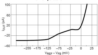
Figure 18. Error Amplifier I<sub>OUT</sub> vs. V<sub>FB</sub>
