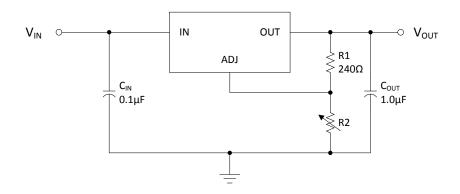
$$V_{OUT} = V_{REF} (1 + R2 / R1) + (I_{ADJ} \times R2)$$
