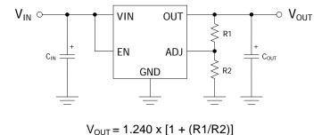
Figure 2. Adjustable Regulator with Resistors
