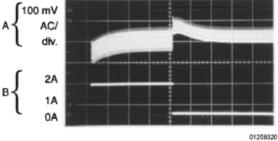
Horizontal Time Base: 200 µs/div. A: Output Voltage, 100 mV/div. (AC)
