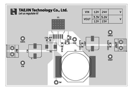
Figure 28. PCB Layout Example
