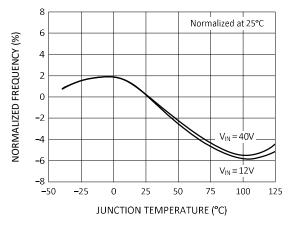
Figure 7. Oscillator Frequency
