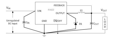
Figure 19. Fixed Output Voltage Version
