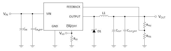
Figure 27. Schematic for PCB Layout Example
