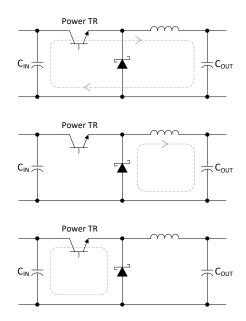
Figure 26. Current Flow in Buck Application
