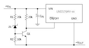
Figure 16. Undervoltage Lockout for Buck-Boost Circuit
