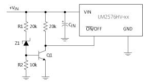
Figure 15. Undervoltage Lockout for Buck Circuit
