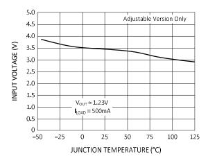
Figure 10. Minimum Operating Voltage
