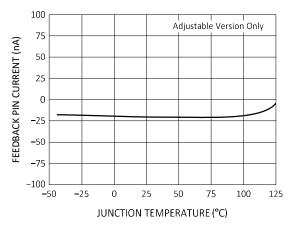
Figure 12. Feedback Pin Current
