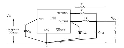
Figure 20. Adjustable Output Voltage Version
