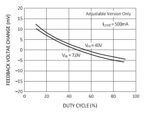
Figure 11. Feedback Voltage vs Duty Cycle
