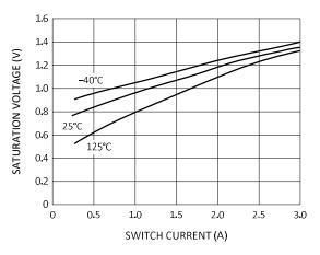
Figure 8. Switch Saturation Voltage
