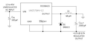
Figure 13. Inverting Buck-Boost Develops -12V
