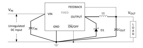
Figure 19. Fixed Output Voltage Version
