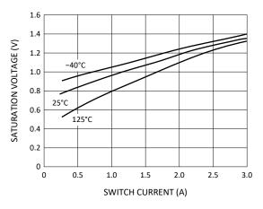
Figure 8. Switch Saturation Voltage
