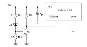
Figure 15. Undervoltage Lockout for Buck Circuit
