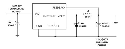
Figure 13. Inverting Buck-Boost Develops -12V
