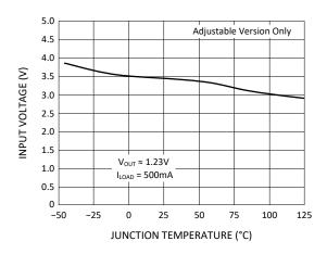
Figure 10. Minimum Operating Voltage
