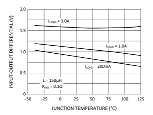
Figure 3. Dropout Voltage
