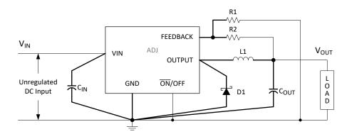
Figure 20. Adjustable Output Voltage Version
