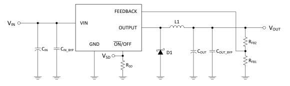
Figure 27. Schematic for PCB Layout Example
