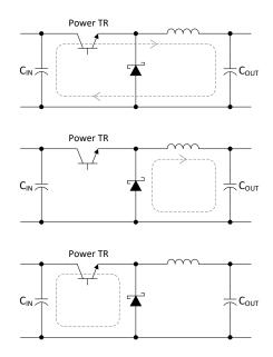
Figure 26. Current Flow in Buck Application
