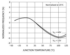
Figure 7. Oscillator Frequency
