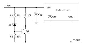
Figure 16. Undervoltage Lockout for Buck-Boost Circuit
