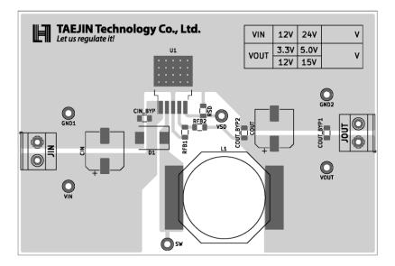
Figure 28. PCB Layout Example
