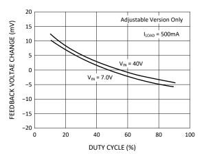
Figure 11. Feedback Voltage vs Duty Cycle
