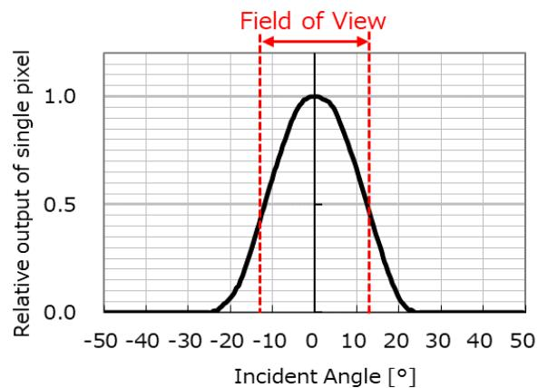
Field of View (FOV): The field of view is defined as angle range obtained 50% or more sensor output relative maximum output.
