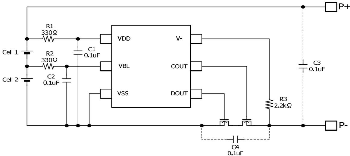
R1 , C1 , R2 , C2 stabilize a supply voltage ripple. However, R1 is enlarged, the detection voltage shifts by voltage when c current consumption flows into R1. Please decide it after confirming the characteristic. Moreover, adjust the value of C1 , C2 to 0.01uF or more to do the stability operation, please.
